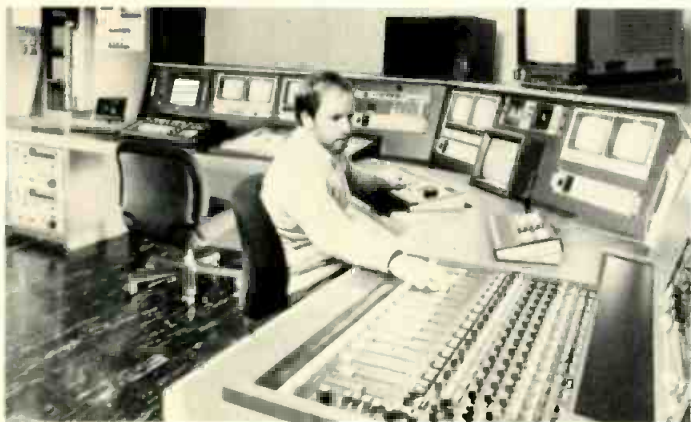
The interformat, rough-cut suite at NFL Films Video is convertible to a full on-line room with Sony BVE-5000.
